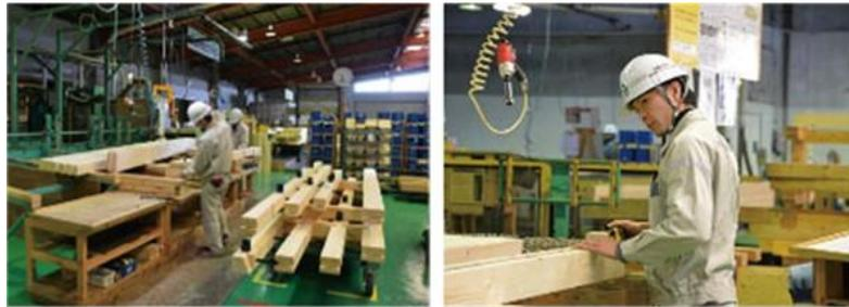
Figure 8 – Yabashi Forestry Co., Ltd. manufacturing pre-cut lumber for construction
